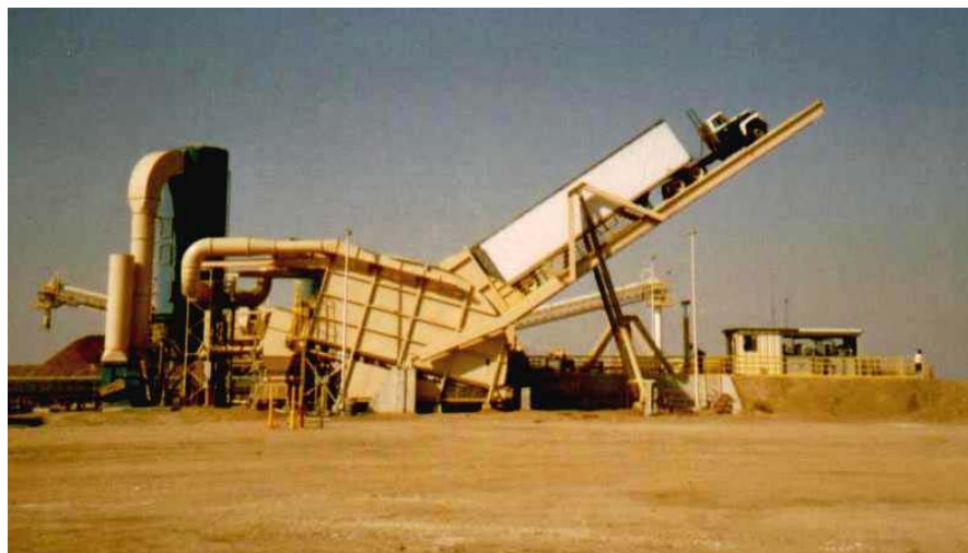
Figure 13. Phelps' truck dump with dust containment
